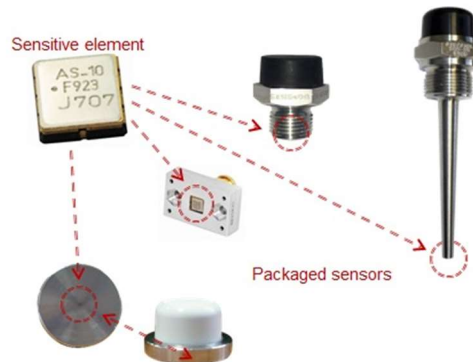
Figure 5. A breakdown of the components in a SAW sensor and the different forms (“How SAW Sensors Operate?,” n.d.).
