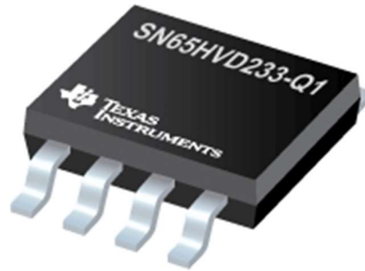
Figure 4. Texas Instrument module for a transceiver addition to the micro-controller ("SN65HVD233-Q1," n.d.).
